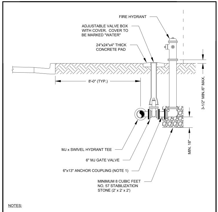
1. LONGER ANCHOR COUPLINGS MAY BE USED WHEN REQUIRED. IF ANCHOR COUPLINGS ARE NOT USED, VALVE SHALL BE RODDED TO THE TEE AND HYDRANT SHALL BE RODDED TO THE VALVE USING A MINIMUM OF TWO (2) 3/4" THREADED RODS ON EACH CONNECTION.
